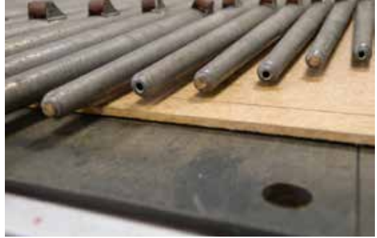
Wood, chewed by insects, blocked up the feet of some of the pipes
